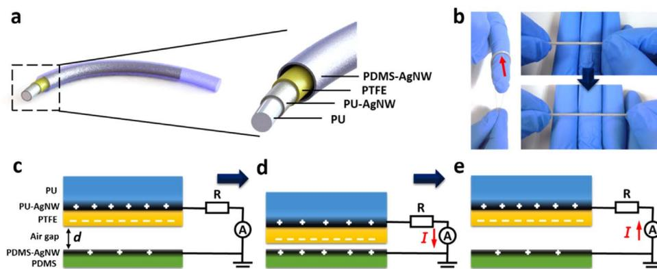
Fig. 1. Schematic illustrations of the FNG structure and the operation mechanism. (a) The structural schematic diagram of the FNG device. The external electric circuiting is omitted for clarity. (b) The photograph of the FNG device wrapping around a finger (marked by the red arrow, left) and being stretched to strain of  $\sim 50\%$  (right). (c–e) The operation mechanism illustration including a cycle of gap size decrease and recover.
