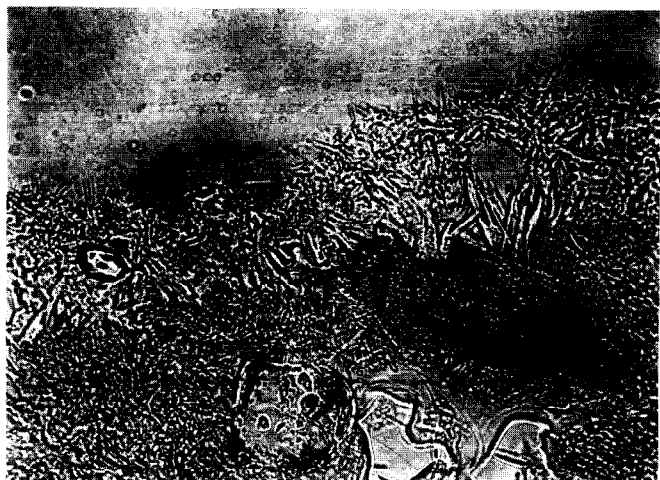
FIGURE 52 - Microstructure of Jun sample, crystallization of anorthite and plagioclase crystals at the body-glaze interface, X 478, transmitted light.
