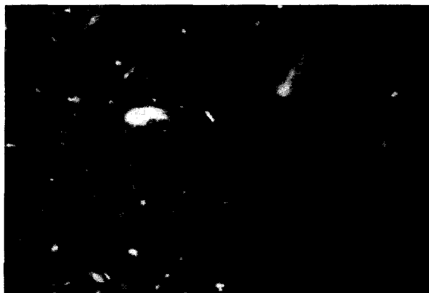
FIGURE 41 - The microstructure of Homudu pottery (7000 years) with included carbonized material.
