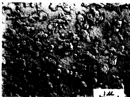
FIGURE 57a - Ji-zhou Tortoise shell, showing its two-phase microstructure.
