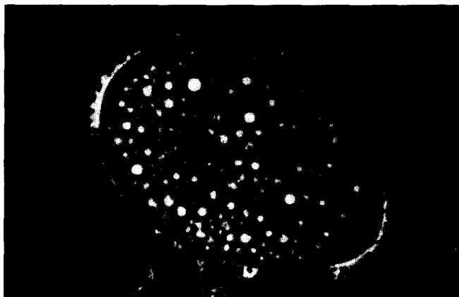
FIGURE 60 - Secondary phase separation seen in the elliptical area, transmitted light, X 742.
