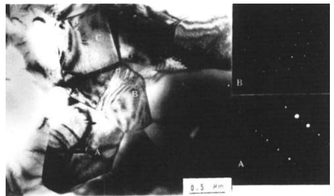
Fig. 4. Electron micrograph of Y-TZP showing three tetragonal grains, A, B, and C, and the diffraction patterns of grain A with [013], of t -phase and [111], of t -phase of grain B.
