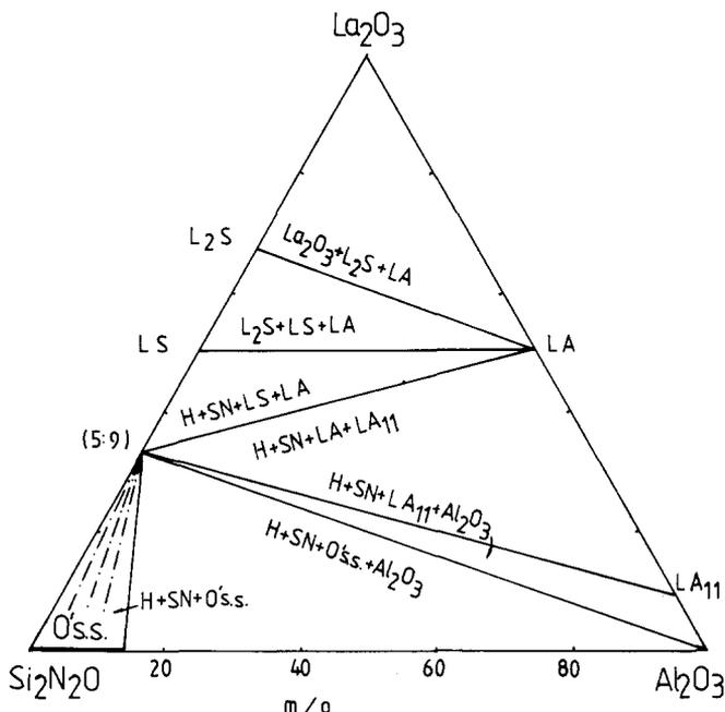
Fig. 2. Sub-solidus diagram of the  $\text{Si}_2\text{N}_2\text{O}-\text{Al}_2\text{O}_3-\text{La}_2\text{O}_3$  system.  $5:9 (5\text{La}_2\text{O}_3 \cdot 9\text{Si}_2\text{N}_2\text{O} = 4\text{Si}_3\text{N}_4 + \text{La}_{10}(\text{SiO}_4)_6\text{N}_2)$ .
