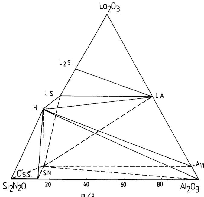
Fig. 1. Sub-solidus diagram of the  $\text{Si}_2\text{N}_2\text{O}$ - $\text{Al}_2\text{O}_3$ - $\text{La}_2\text{O}_3$  system.  $\text{L}_2\text{S} = 2\text{La}_2\text{O}_3 \cdot \text{Si}_2\text{N}_2\text{O}$ ;  $\text{LS} = \text{La}_2\text{O}_3 \cdot \text{Si}_2\text{N}_2\text{O}$ ;  $\text{LA} = \text{La}_2\text{O}_3 \cdot \text{Al}_2\text{O}_3$ ;  $\text{H} = \text{La}_{10}(\text{SiO}_4)_6\text{N}_2$ .
