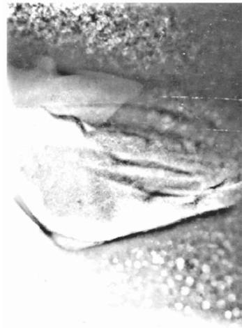
(b) Interconnected and droplet phase separation structures coexist, resulting from local chemical variation
