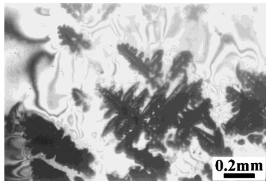
Fig. 1. Regular dendritic growth of 0.76PMN–0.24PT crystals on {001} plates, coarser branches outgrowing at an angle of  $90^\circ$  to trunks.
