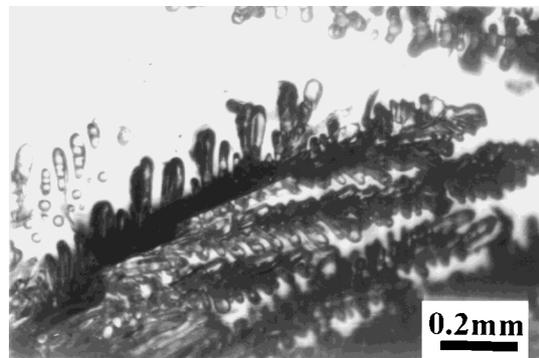
Fig. 2. Irregular dendritic growth of 0.76PMN–0.24PT crystals on {001} plates, the crossed angle of branches deviates from  $90^\circ$ .
