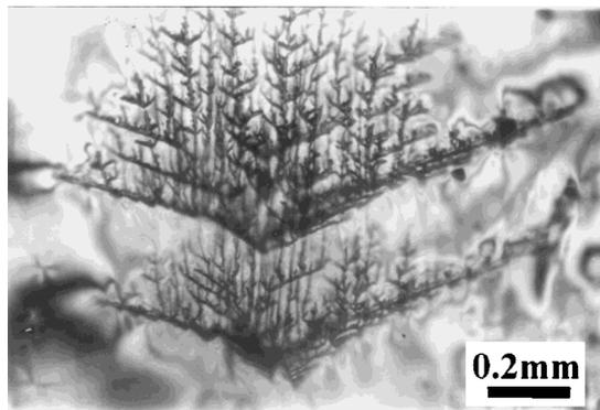
Fig. 3. Typical and perfect crystal trees made up of fine grained PMNT crystallites.
