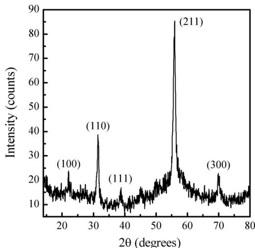
FIG. 1. XRD pattern of the grain-oriented PMN-0.3PT ceramics, where the measured surface was perpendicular to the solidifying direction.
