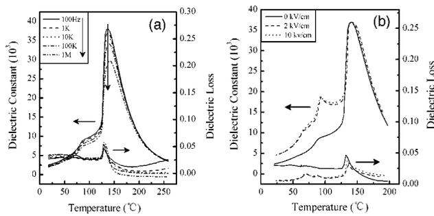
FIG. 2. Temperature dependence of dielectric constant and loss tangent (measured upon heating) of the  $\langle 112 \rangle$  grain-oriented PMN–0.3PT ceramics (a) for an unpoled sample at various frequencies, and (b) for a sample poled under dc fields of 0 kV/cm, 2 kV/cm, and 10 kV/cm at 1 kHz.
