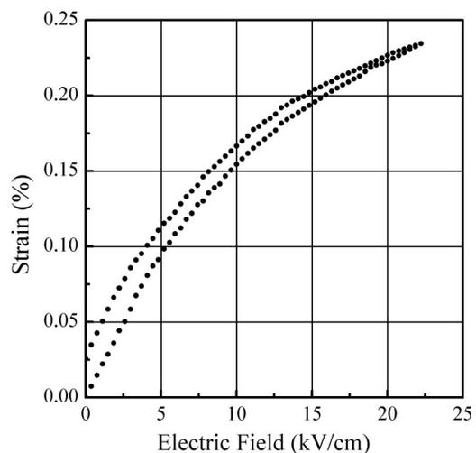
FIG. 4. Strain vs electric-field curve for the  $\langle 112 \rangle$  grain-oriented PMN–0.3PT ceramics.
