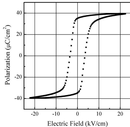
FIG. 3. Polarization vs electric-field hysteresis loop for  $\langle 112 \rangle$  grain-oriented PMN–0.3PT ceramics.
