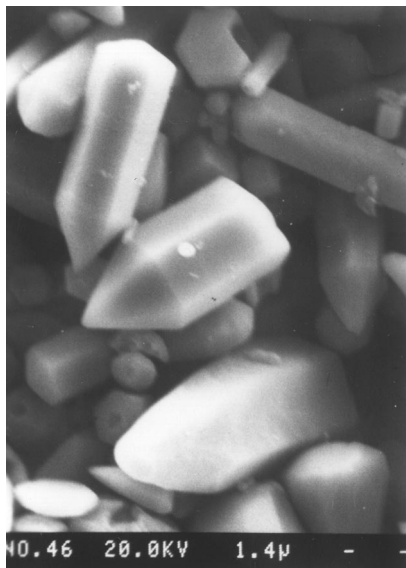
Fig. 2. SEM micrograph of powder prepared by hydrothermal salt solution pressure-relief using 0.5 mol/l Zn(CH_3COO)_2 solution as precursor at 250°C.
