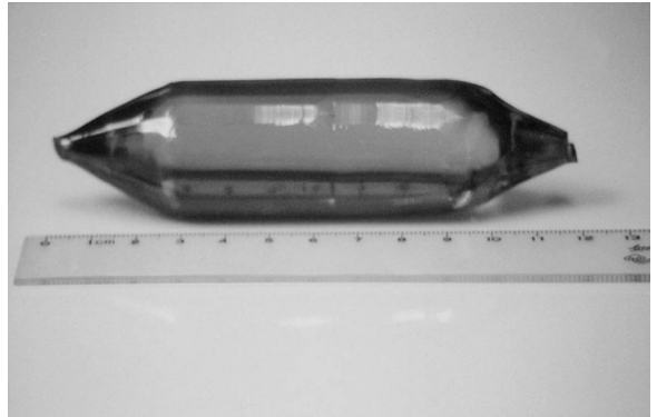
Fig. 1. 30 at% Yb:YAG crystal boule grown along the \langle 111 \rangle direction.
