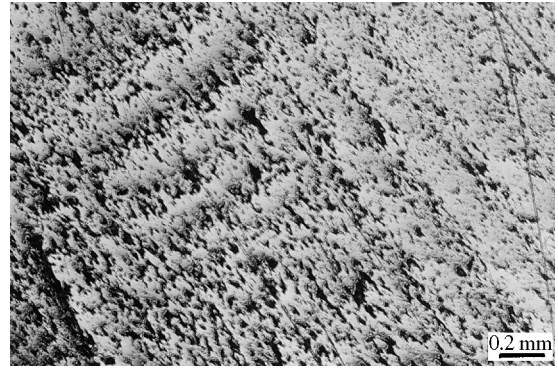
Fig. 3. Pores in PMNT 67/33 crystals under polarizing microscope.
