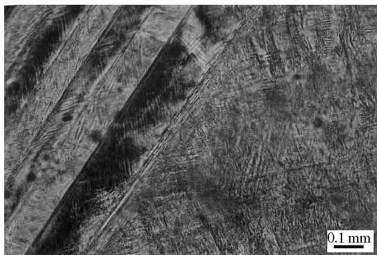
Fig. 1. Nonuniform distribution of domains in PMNT 67/33 crystals under polarizing microscope.
