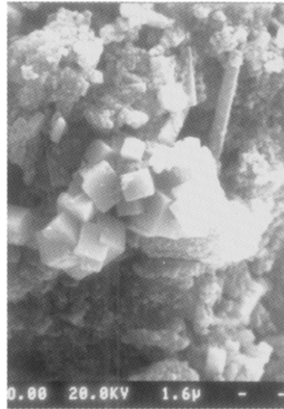
Fig. 7. SEM photograph of \text{CaF}_2 crystallites prepared by using \text{CaSO}_4 and \text{NaF} as precursors at 200^\circ\text{C} .
