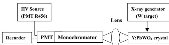
Fig. 7. Scheme of the setup for measuring the radioluminescence emission spectra of Y:PbWO<sub>4</sub> crystal.
