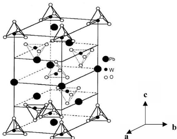
Fig. 1. Structural diagram of unit of scheelite-structured  $\text{PbWO}_4$  crystal.
