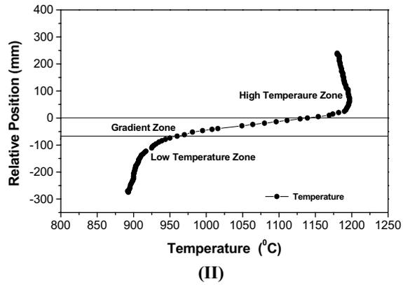
Fig. 2. Schematic (I) and temperature profile (II) of crystal growth furnace.
