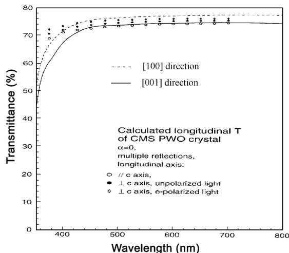
Fig. 6. Comparison between theoretical and experimental transmittance curves of Y:PbWO<sub>4</sub> crystal along the [100] and [001] directions.
