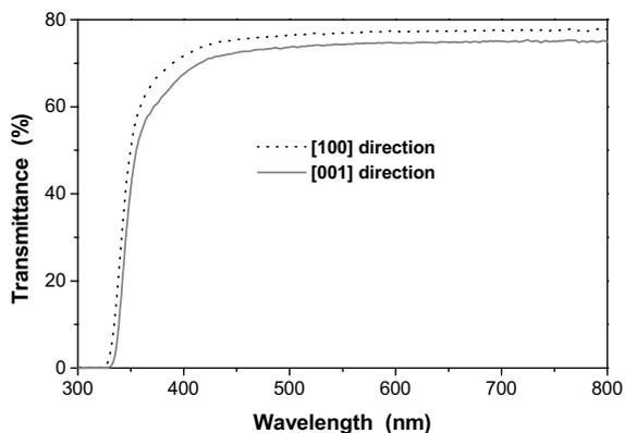
Fig. 5. Transmittance spectra of Y:PbWO<sub>4</sub> crystal along the [100] and [001] directions.
