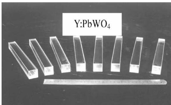
Fig. 3. Full-size Y:PbWO<sub>4</sub> crystals (length: 230 mm) for the CMS grown by the modified Bridgman method.
