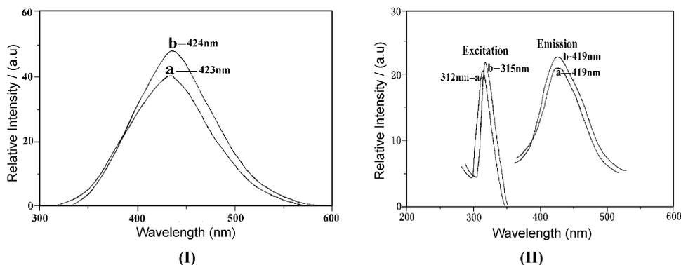
Fig. 8. Radioluminescence emission spectra (I) and photoluminescence emission spectra (II) along (a) [1 0 0] and (b) [0 0 1] directions of Y:PbWO<sub>4</sub> crystal.
