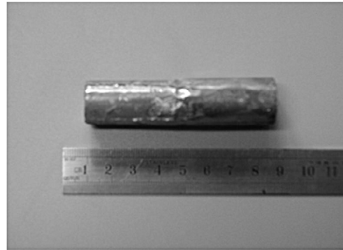
Fig. 2. As grown PMINT single crystal boule by the modified Bridgman technique.
