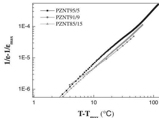
Fig. 2. Plot of  $\log(1/\epsilon - 1/\epsilon_{\max})$  vs  $\log(T - T_{\max})$  of the (1-x)PZN-xPT single crystals.
