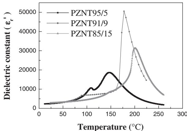
Fig. 3. Temperature dependence of the dielectric constant of the poled  $(1-x)\text{PZN}-x\text{PT}$  crystals (001) planes at 1 kHz upon heating.
