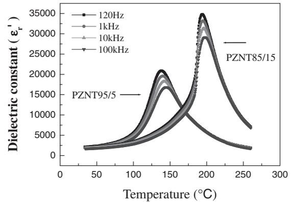
Fig. 1. Temperature dependence of the dielectric constant measured at different frequencies upon heating of the (1-x)PZN-xPT crystals (001) planes.
