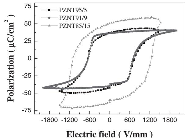
Fig. 4. Electric hysteresis loops of the  $(1-x)\text{PZN}-x\text{PT}$  crystals (001) planes.
