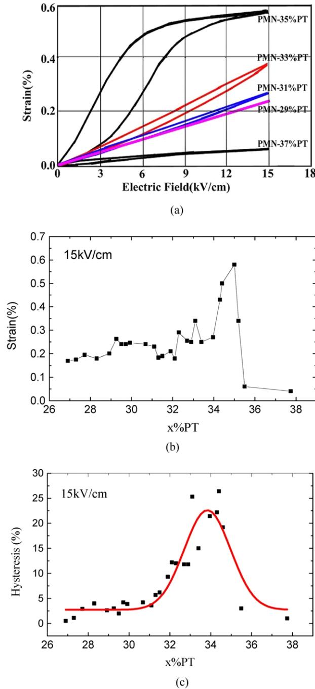
Fig. 1. (a) Strain versus  $E$ -field (unipolar,  $E \leq 15$  kV/cm) curve for  $\langle 001 \rangle$  oriented PMNT crystals. Strain and hysteresis as a function of PT content ( $x\%$ ) for  $\langle 001 \rangle$  oriented PMNT crystals in (b) and (c), respectively. Solid line in (c) represents the gauss fits to strain hysteresis.
