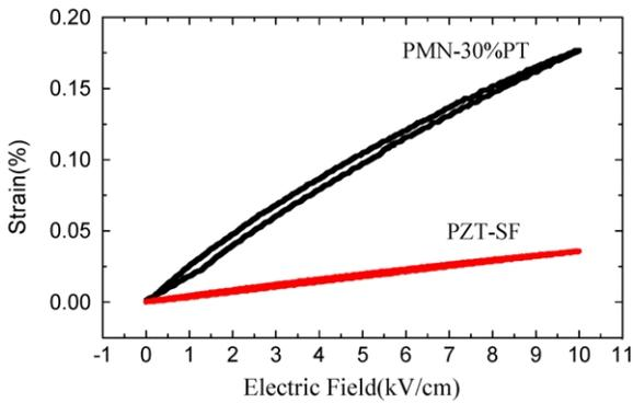
Fig. 2. The strain behavior for PMN-30%PT crystals and PZT-SF ceramics at the same drive  $E$ -fields.
