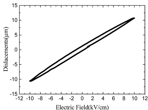
Fig. 5. Strain versus electric field characteristics for PZT-SF multilayer actuators.
