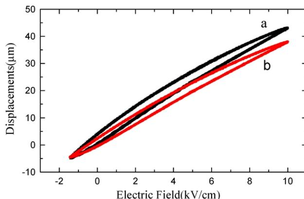
Fig. 4. Strain versus electric field characteristics for PMNT multilayer actuators (a) free-loading (b) 4 kg loading.
