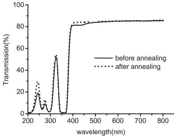
Fig. 2. Optical transmission spectra of the yellowish LSO:Ce before and after annealing.
