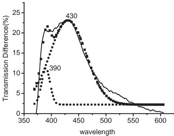
Fig. 5. Difference spectrum between the transmission spectra of the damaged LSO:Ce crystal before and after irradiation and its Gauss fitting.
