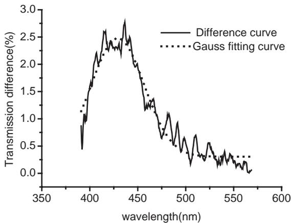
Fig. 3. Difference between transmission spectra before and after annealing and Gauss fitting for yellowish LSO:Ce sample.
