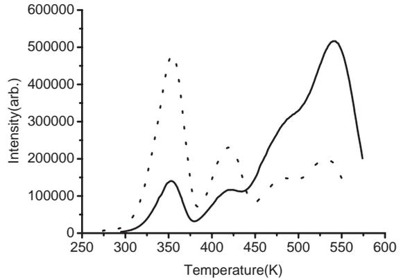
Fig. 7. Thermoluminescence spectra of the radiation-damaged LSO:Ce crystal before (dotted line) and after  $\gamma$ -ray irradiation (solid line).
