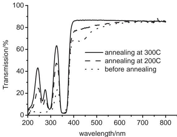
Fig. 8. Transmission spectra of the radiation-damaged LSO:Ce crystal before (dotted line) and after annealing at 200°C (dashed line) and 300°C (solid line).
