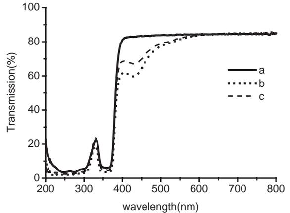
Fig. 4. Optical transmission spectra of LSO:Ce crystals after  $\gamma$ -rays irradiation. Curves *a* and *b* are for two different conditions of colorless crystals. Curve *c* is for the originally yellowish crystal.
