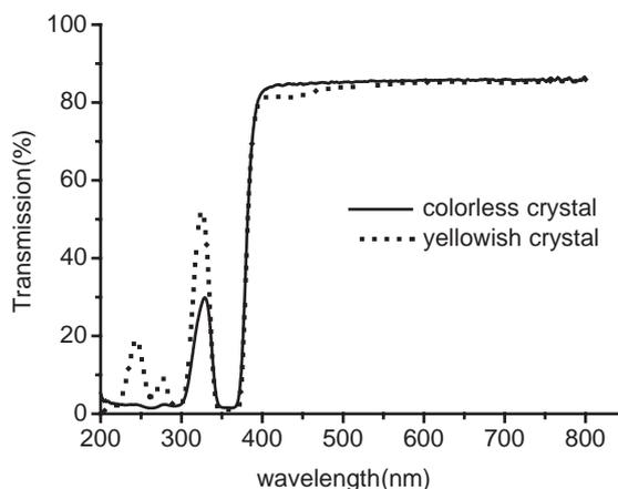
Fig. 1. Transmission spectra of the as-grown colorless and yellowish LSO:Ce crystals.
