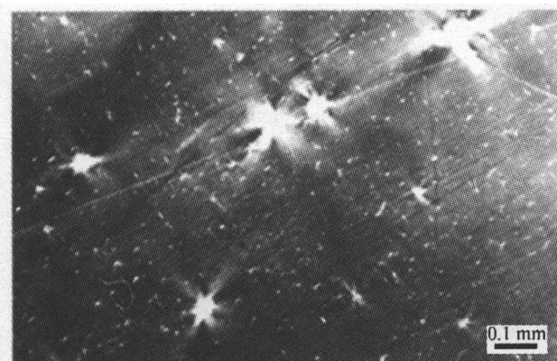
Fig. 6. The scattering particles in PMNT crystals observed under crossed polarizing microscopes.
