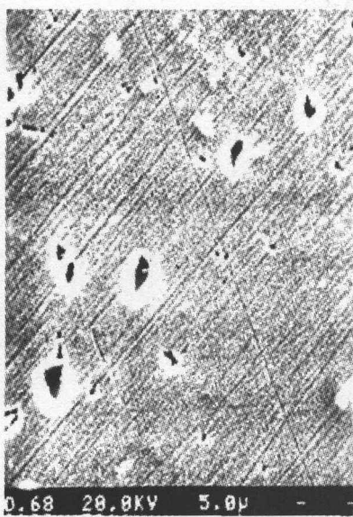
Fig. 7. The pores in PMNT crystals under SEM.
